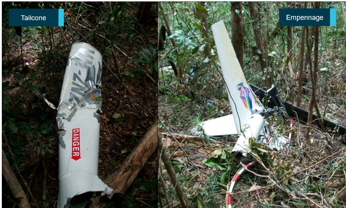
Figure 7: Separated tailcone (left) and empennage (right)
