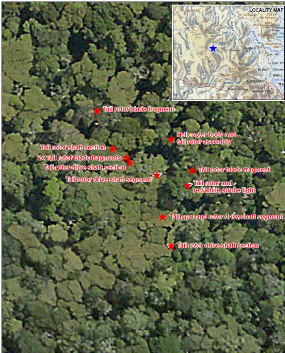
The distribution of the wreckage, as mapped by Queensland Police Service. The item marked 'Tail spar and rotor drive shaft segment' refers to the tailcone with the seized section of tail rotor driveshaft inside.
